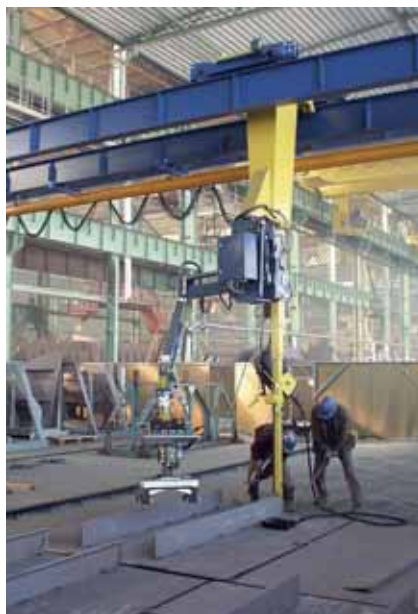
Stiffener profiles are assembled semi-automatically on Baltija Shipbuilding Yards panel production line in Lithuania.
