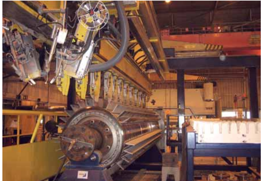
Fin profile assembly- and welding portal above a work-piece attached to a rotation- and support roller bed. Profile cassette on the right.
