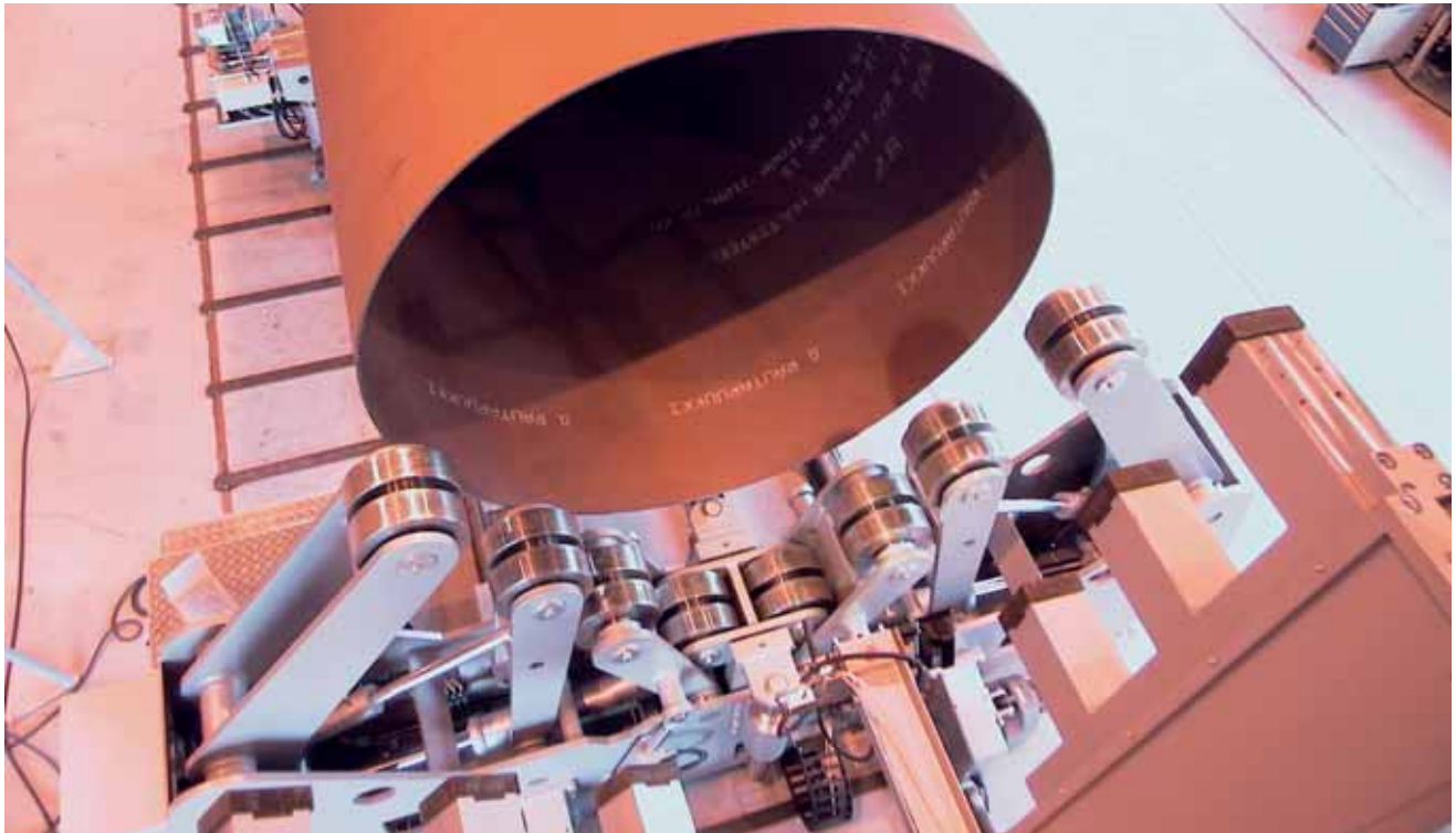
A windmill tower section is moved to a hydraulic jig.
