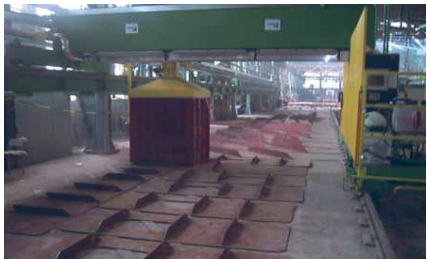
Work area of Vision welding robot at the 4 x 12.5 m panel line at the 3rd May Shipyard.
