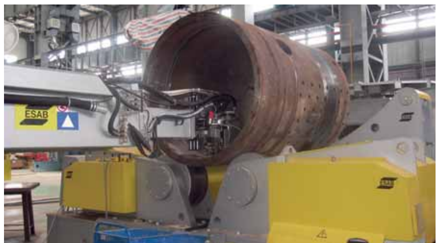
Narrow gap welding using a column & boom and heavy roller bed at the factory of Dong Fang Heavy Machinery.
