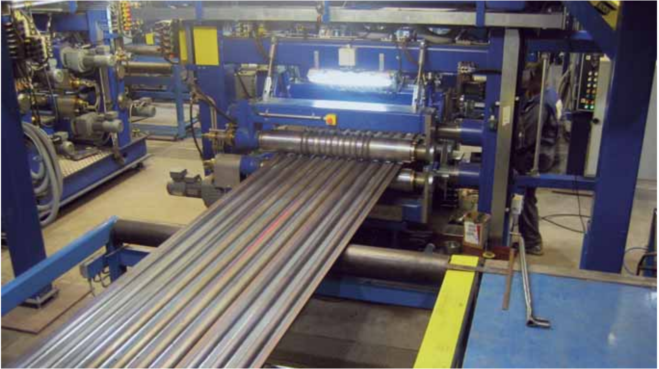
Membrane wall-panel being manufactured on Rafako's new welding line.
