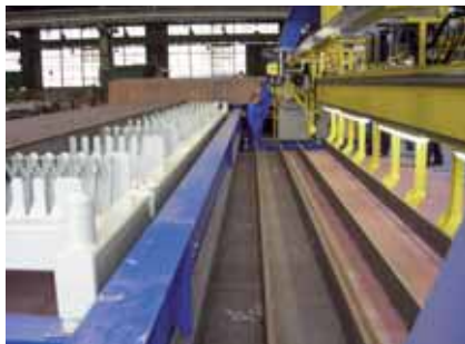
Assembly of stiffener profiles at the Naval Yard's thin plate line in Poland.
