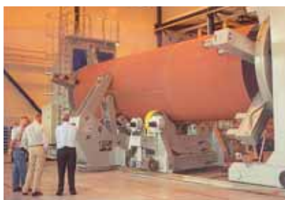
Tower sections attached to a PEMA head and tailstock system.
