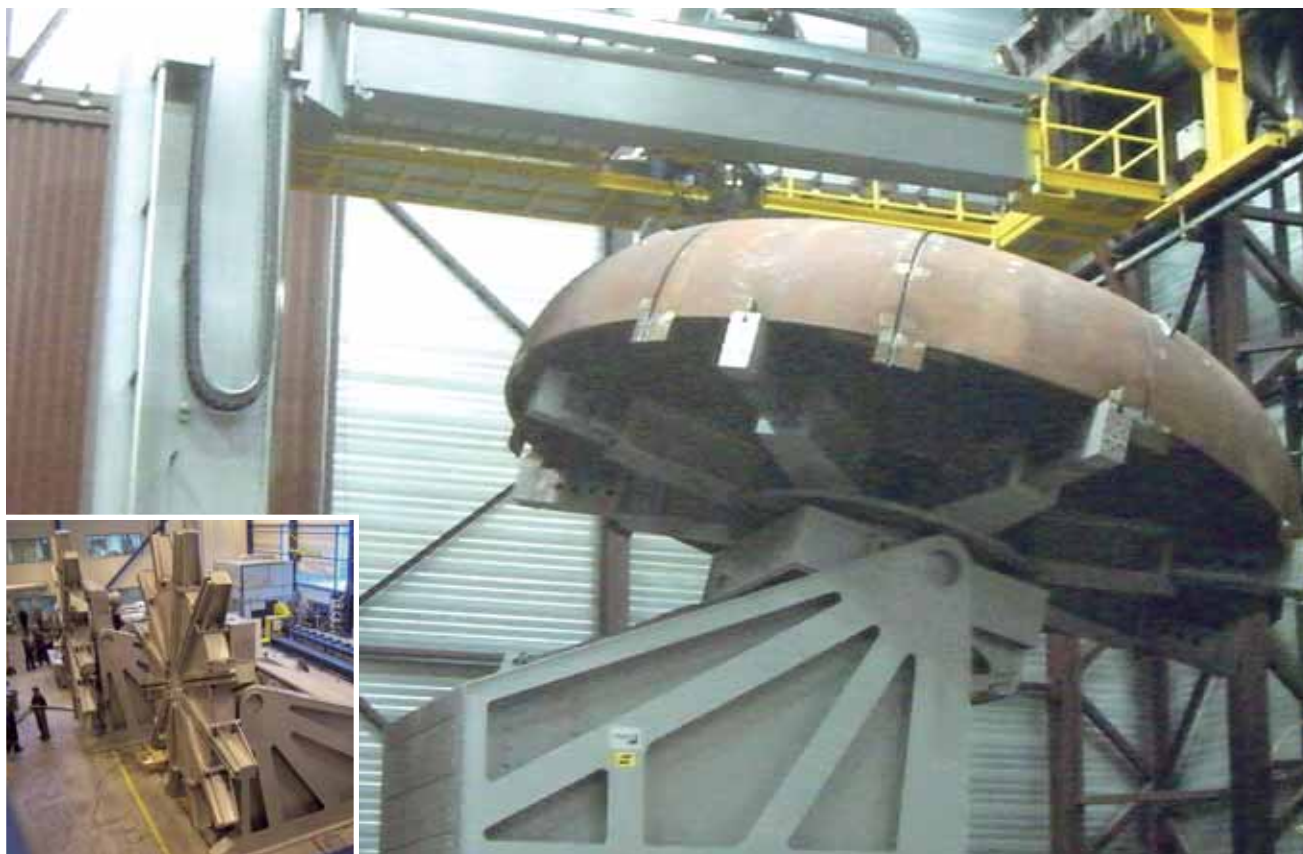
A heavy column & boom/work-piece handling station belonging to COEK Engineering of Belgium. In the small picture, Gigantic 120-tonne positioners awaiting transportation to China.
